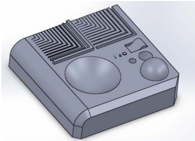
FIGURE 2. Prototype model of a test part to characterize printed surface flaws.
